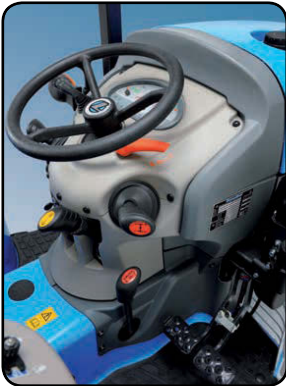
2 Series. Ergonomic gearshift levers.
