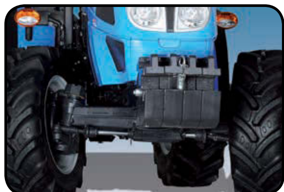
Front axle. 55° steering angle.
