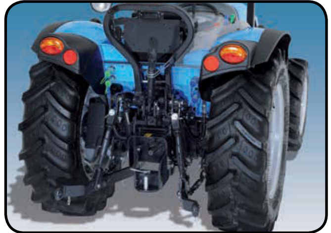
Rear power lift. 1,200 kg lifting capacity.
