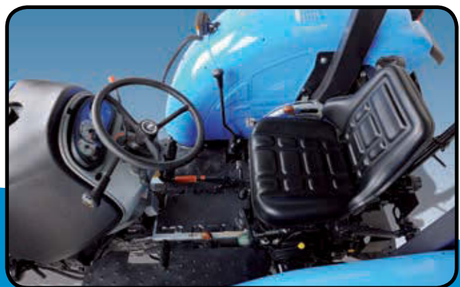
Driver's area. Improved ergonomics with gearshift levers now positioned at the side.
