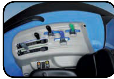
Right control panel: Power lift and control valve levers.
