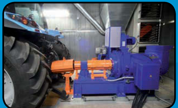
R&D Center. The new test rooms for transmissions and engines.
