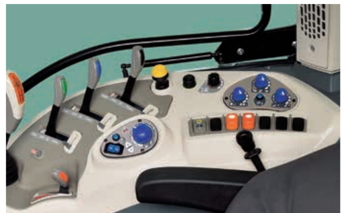
HYDRAULICS. Ergonomic controls for the electronic hitch and hydraulic control valves are on the console on the driver's right.
