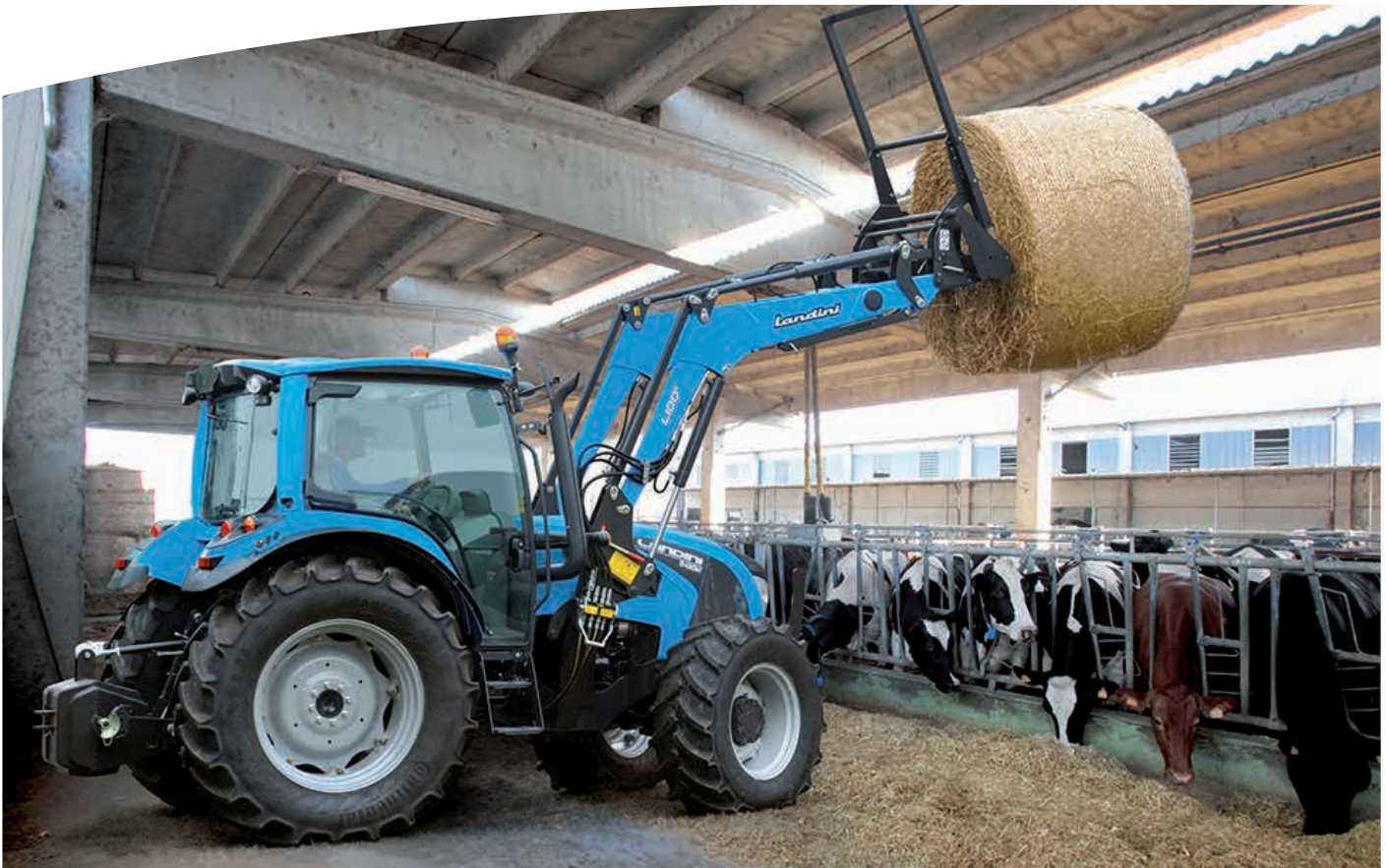
L SERIES. An L100 front loader at work in a livestock farm.
