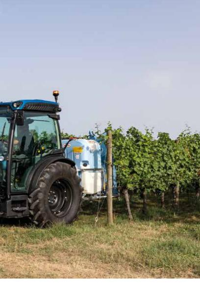
The F and S versions are fitted with either 24- or 28-inch rear tyres. For the GT version, 24-inch, 28-inch extra-wide and 30-inch oversized tyres are also available to suit widely spaced orchards and open field applications.
