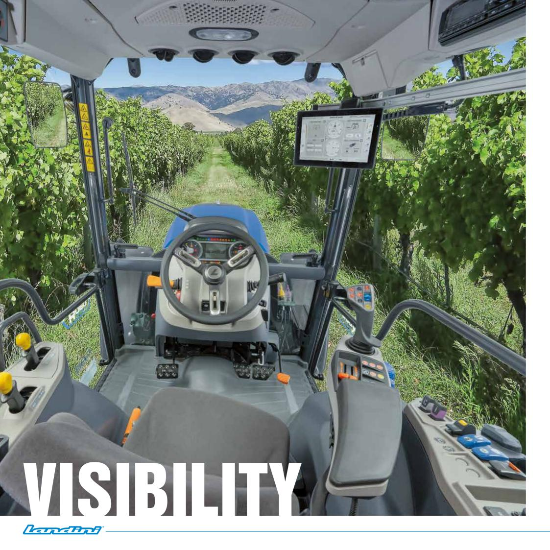
The cab of my **REX4** offers unobstructed vision in all directions, so I always keep my implements in view. And the cab suspension and the flat-deck platform ensure a smooth, comfortable ride in any situation. And the filtration system? Absolutely perfect! So now I can carry out pest control treatments in complete safety...
